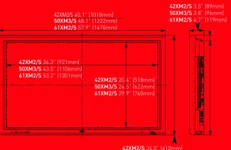
42XM2/S 24.0" (610mm) 50XM3/S 29.0" (736mm) 61XM2/S 34.6" (880mm)
